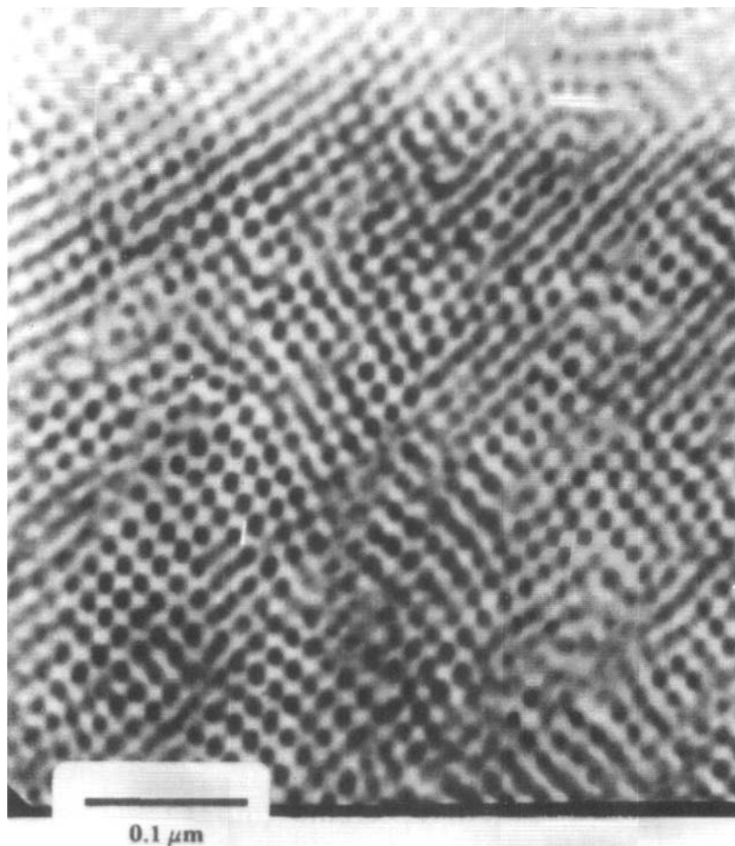
FIG. 17. Transmission electron micrograph of a PS-PIB-PS block copolymer synthesized at -80^{\circ}\text{C} in 60/40 hexane/methyl chloride, using an IB reaction time corresponding to 91% IB conversion.
